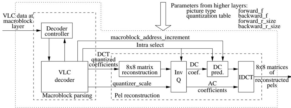
Figure 1. Macroblock parsing and pel reconstruction module – adapted from [5].
