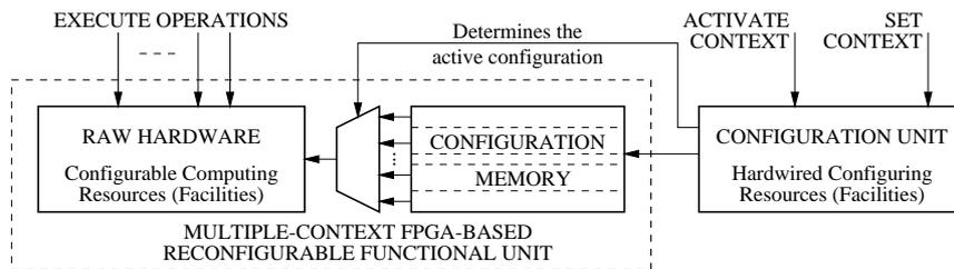
**Figure 2.** The organization of the RFU and associated configuration unit.
