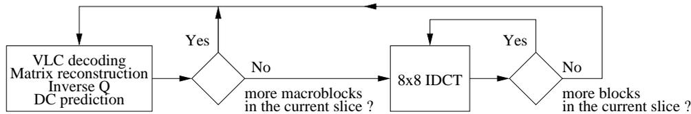
**Figure 4.** The computing scenario of the macroblock parsing and pel reconstruction routine.
