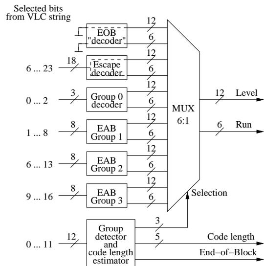
**Figure 3. The VLD implementation on FPGA.**
