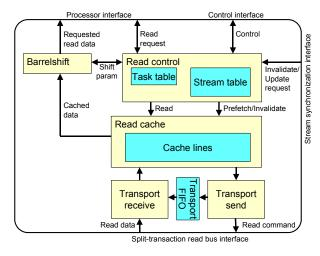
Figure 4. Read unit inside the processor shell.
