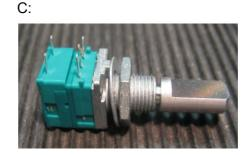
Type A, produced by DDM, is Conrad art.nr. 705594-89, which I have used for a long time already, and for which the PCB footprint was designed. It lacks a facility to screw it into a front plate. I only recently discovered type B in the Conrad catalog, art.nr. 700697-89. This switch from Alps (type STEC11B03) seems a better choice: its clicks feel smoother, and the metal housing and shaft have a better fit, more suitable for heavy control knobs.
