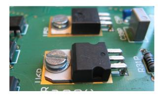
As exception to the 'normal' mounting order, prior to mounting the 4 op amps and the 2 micro controllers: complete all mounting except these 6 IC's and the XLR connectors. We can now first test the correct operation of the power supplies before inserting these IC's, avoiding the risk to blow them due to some earlier mistake. So, without the 4 op amps and 2 micro controllers U1D and U2D, you connect the two transformers, and power them up. Now the following voltages must be checked:
