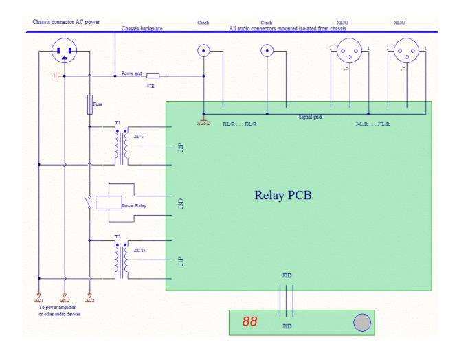
If you intend to switch a heavy transformer of a power amplifier, it is probably a good idea to add a 'varistor' across the primary side of the transformer. A varistor will prevent that switching-off the transformer creates a high-voltage arc across the relays contacts. The varistor will thus help in maintaining a proper lifetime of the relay. In any case, I would select a significantly over-powered relay, to obtain a trouble-free and very long lifetime.
