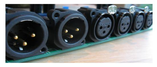
If you want to equip the preamp with 3 pair of XLR inputs plus 3 pair cinch inputs, diode D4D should NOT be mounted. Alternatively, if you want 2 XLR inputs and 4 cinch inputs, do insert D4D, and connect the 4<sup>th</sup> cinch pair to the pins marked with '+' on J4L and J4R. As in the regular use of XLR connectors for audio, the output connectors are 'male' (have pins), and the input connectors are 'female' (have holes).
